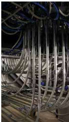
Via long pipe systems plastics are injected with compressed air into the blast furnace.
