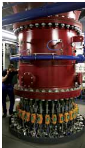
Via long pipe systems plastics are injected with compressed air into the blast furnace.
