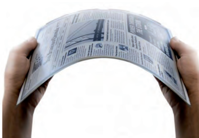
Figure 4. Innovative applications in the electronic sector: a flexible AMOLED screen
