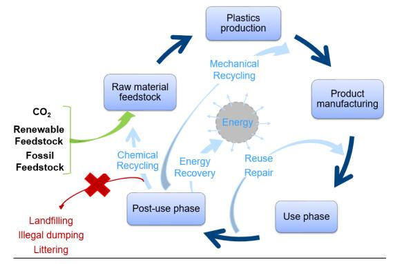
Figure 1: Schematic view: life cycle of products (e.g. packed goods, cars, buildings ...) containing plastics
