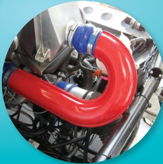
The heat-stable charge air duct replacing the metal part weighs only half as much.
