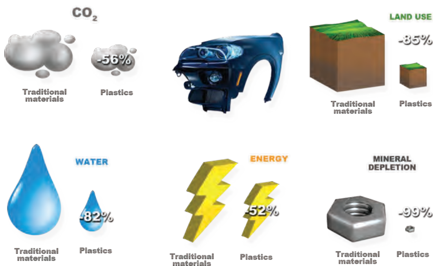
Resource efficiency of plastics in the automotive sector Fender case study: plastics versus traditional materials
