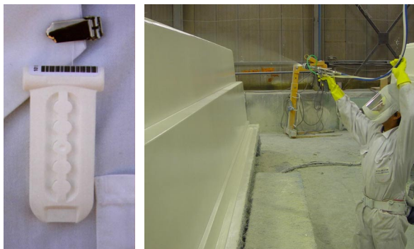
Left: styrene monitoring badge. Right: full protective clothing, including a ventilated breathing system, is worn for the gelcoating of this mould.
