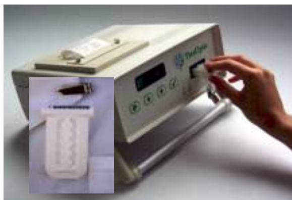
Badge monitoring and data analysis system for recording workplace styrene exposure
