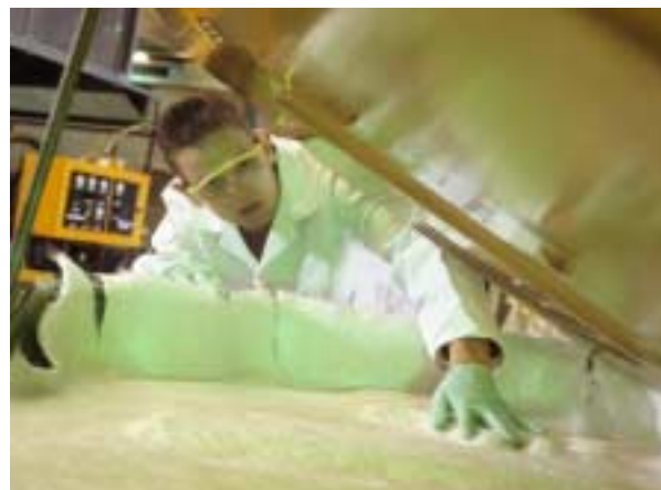
Styrene emission can be substantially reduced by switching to closed moulding techniques like resin infusion (above) or resin injection (below).
