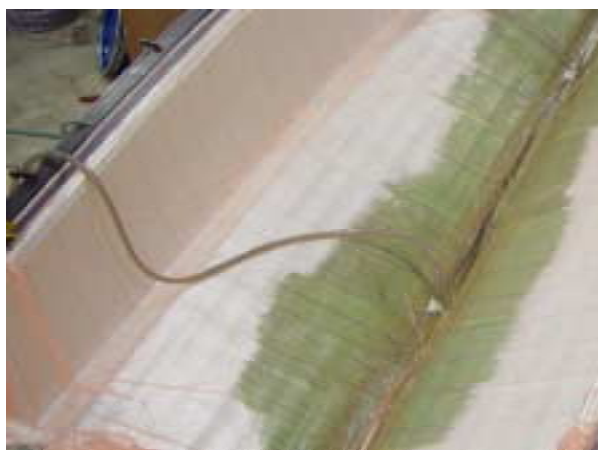
Styrene emission can be substantially reduced by switching to closed moulding techniques like resin infusion (above) or resin injection (below).
