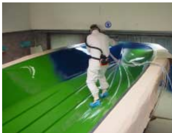
These boat hulls are produced by vacuum infusion with an LSC gelcoat first applied to the open mould.
