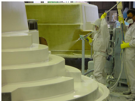
Personal protection equipment being used in an open mould spray operation.
