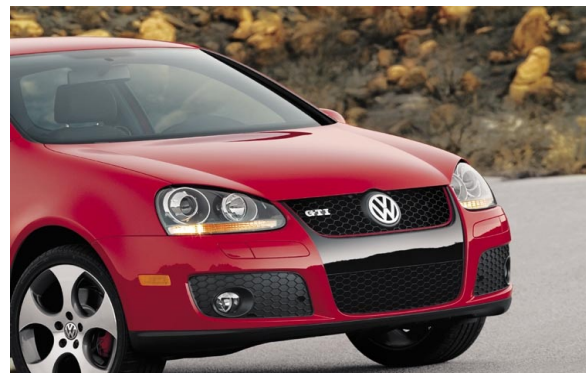
FRP enables attractive and complex shapes to be moulded. Coefficient of expansion is similar to steel so a good panel fit is assured.
