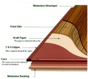
The diagram above shows a cross section of laminate flooring and is a good example of 'wood and plastic lamination' as defined in the Directive. Here a melamine resin is used to provide a protective coating to the wood based core in a distinctive build-up of layers. By contrast, in the FRP lamination process (below), the resin completely 'wets out' the glassfibre to form an integrated and homogenous structure.
