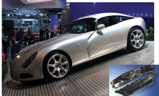
Above: The UK built TVR 350 like many other exotic sports cars, has an FRP monocoque body shell. Lower weight means increased performance and improved fuel economy.
