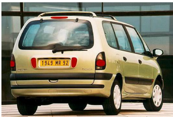
The Renault Espace is a vehicle that has made extensive use of FRP composite body parts throughout its long history.
