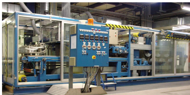
Highly automated processes are used for producing SMC/BMC compound from UP resins and for moulding (converting) the material into finished parts typically used in the automotive and electrical / electronic industries.
