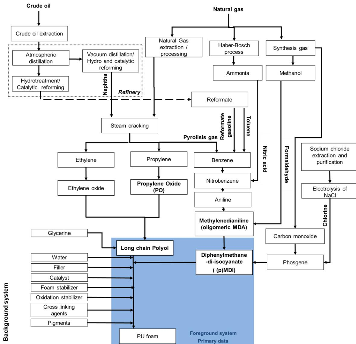
Figure 4: Cradle-to-gate system boundaries MDI based Flexible PU Foam
