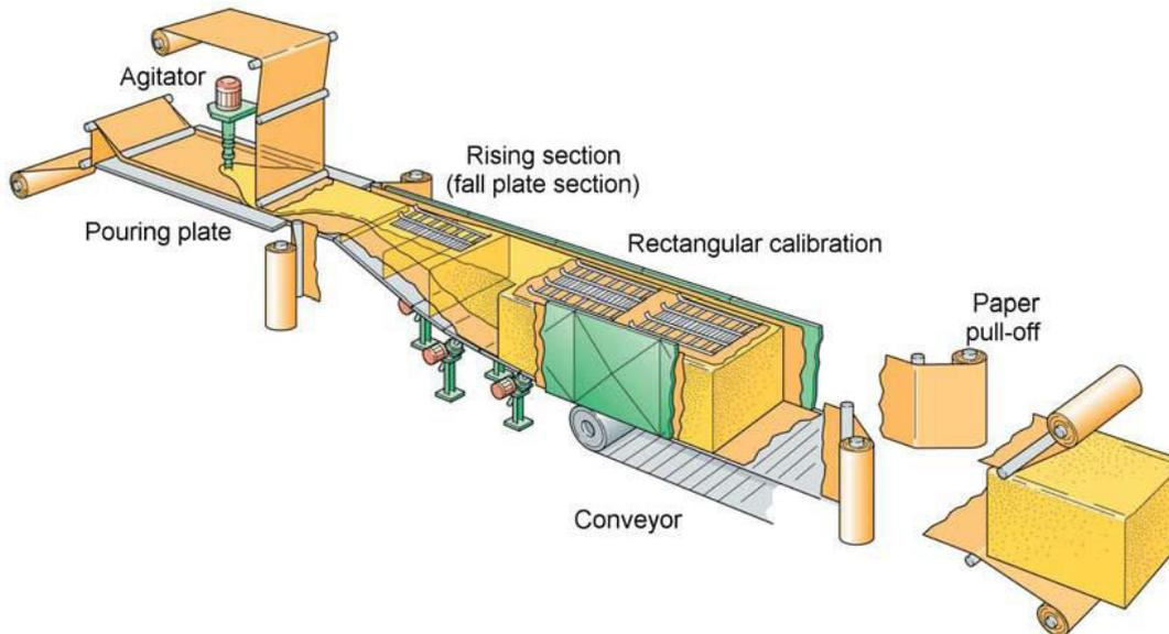
Figure 1: 3-D representation of a system – without metering device and cut-off saw – for continuous production of flexible rectangular foam blocks by means of the QFM process (source: Hennecke GmbH)
