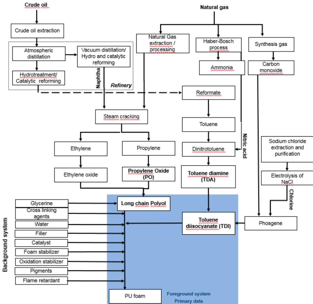
Figure 3: Cradle-to-gate system boundaries TDI based Flexible PU Foam
